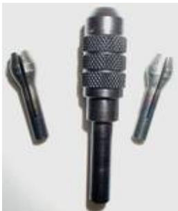
Diagram 1: Common 3 pc Pin Gage Clamping System
